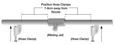
Use the hose clamps to attach the misting hose to the wall or beams.
