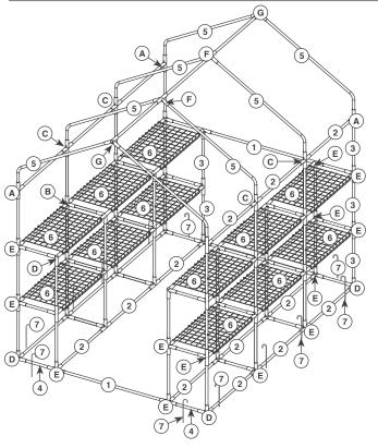
Assemble frame as shown. Metal tubes ①-⑤ push into plastic parts A-G and shelves 6 sit on the horizontal tubes.
