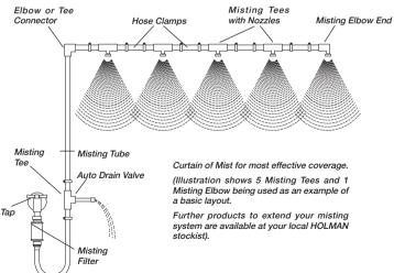
Work out the spacing of the misting jets and cut the misting hose to length and install the relevant misting tees. Finish each line with a misting elbow.
