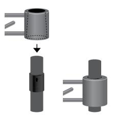
Slide the wire frames onto the clips. The attachments have a slight v-shape. The wider part has to point downwards.
