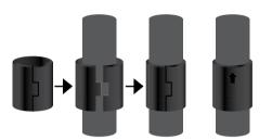
Use the clips to attach the wire frames onto the poles. Clip them onto the pole and lock them into position (grooves). Make sure that the arrows are pointing upwards.
