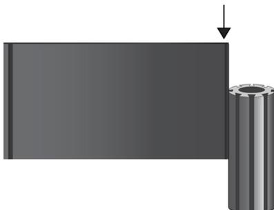
2) Slot the panels in the pillars with the tongue facing up.
