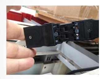
Before you start to remove any displays you will need to locate the cable to the displays and disconnect this. It easily pulls apart and as you would of already switched off the power there is no chance live lines.
