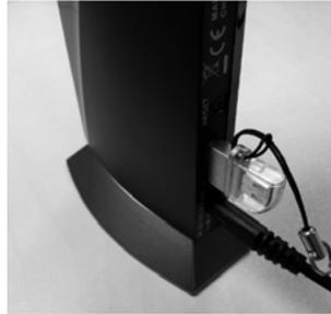
3. Reconnect the **Main Console** DC power to start the firmware update process. During the update process the status LED on the bottom side will flash red.
