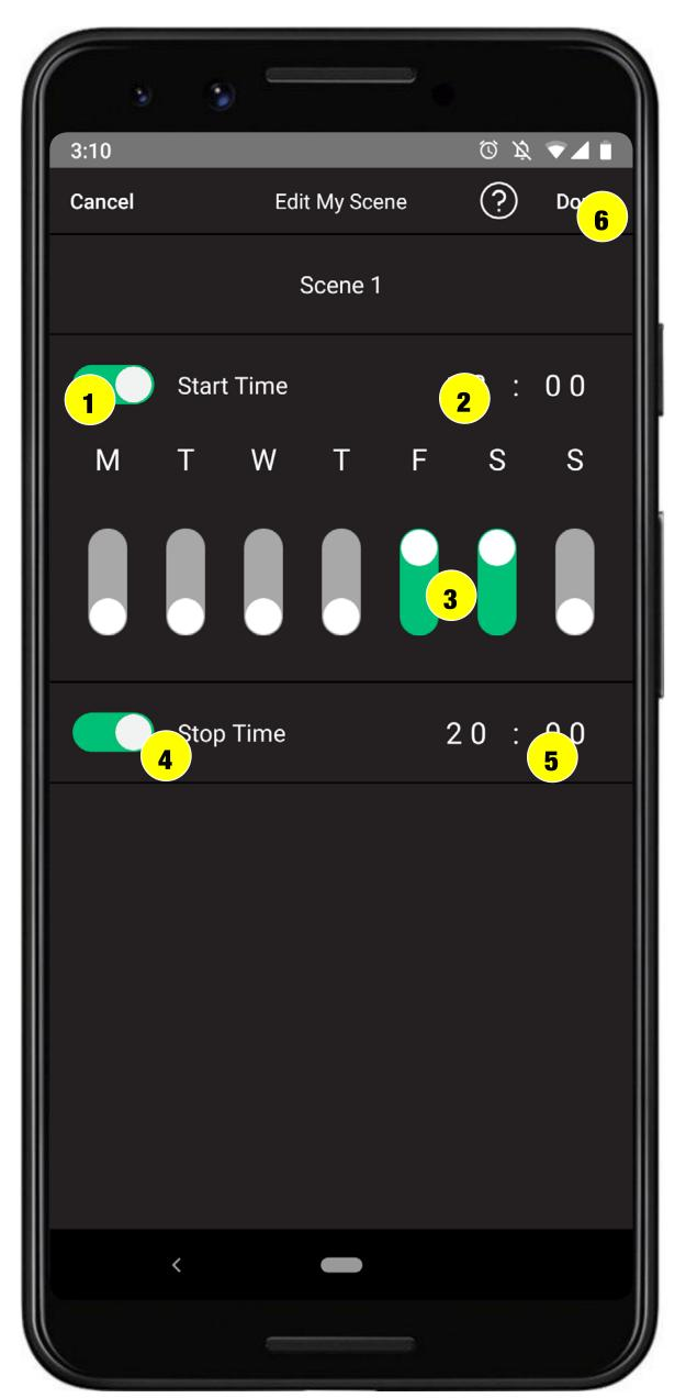
6. When you have finished press **Done**, located at the top of the scene, you can then select off the lights will now run their programmed scene (if you see a red clock with a cross through it under your dimmer bar the controller has not received the program – go closer open the scene and hit done again, when the clock is cleared you can then select off.)
