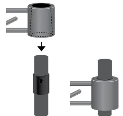
Slide the wire frames onto the clips. The attachments have a slight v-shape. The wider part has to point downwards.
