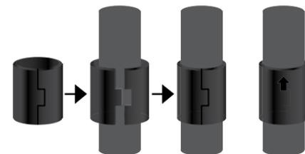
Use the clips to attach the wire frames onto the poles. Clip them onto the pole and lock them into position (grooves). Make sure that the arrows are pointing upwards.
