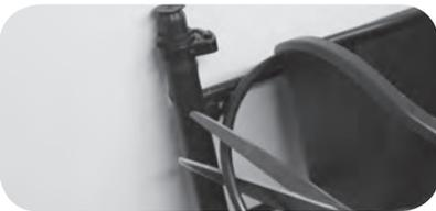
h) Cut the 4mm tube to the length to position the take off in the centre of the pot.
