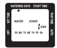
Interval scheduling allows an interval program between (1 to 7 days). Setting a schedule for every 3 days would mean that the tap timer will run every 3 days.
