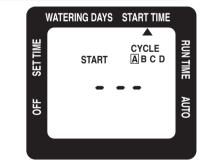
'Start Time' is the time of day that the tap timer will begin watering. You can set up to 4 cycles (start times).
