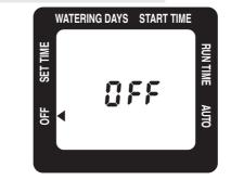
'OFF' mode is used to stop watering for an extended period of time. Press ( ) untill the arrow is pointed to 'OFF'.
