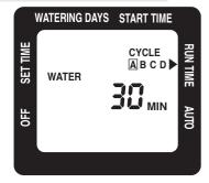
'Run Time' sets the length of time that the cycle will water for. You can set a different run time per cycle.
