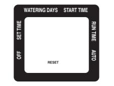
• Press and hold (0K) for 5 seconds to erase all settings in the timer and it will return to the original factory settings. The screen will display RESET.
