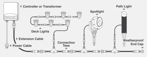
Only use lights within one colour system, either RGB Colour 4-Pin Plug + Socket or Warm White 2-Pin Plug + Socket
