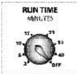
Note: To continue the automatic watering schedules, move the *Run Time* dial into one of the preset *Run Time* positions.
